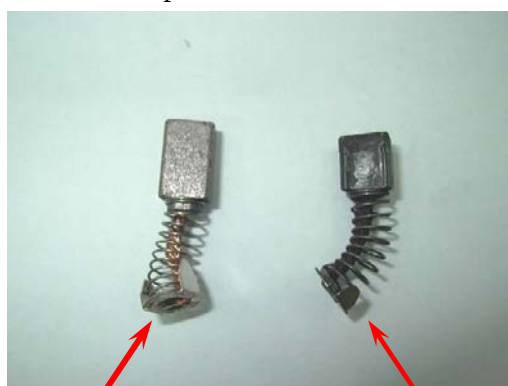
New Motor Brush Worn Motor Brush
