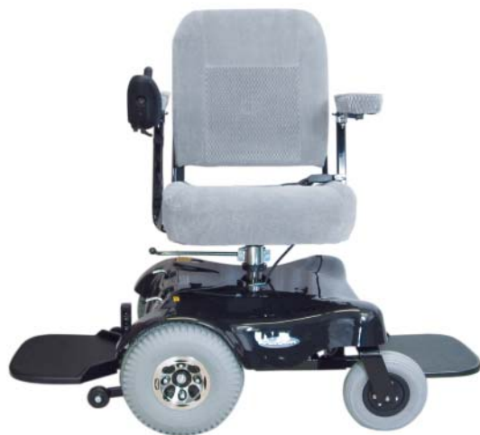
Convertible with Dual Footplates Height, Length & Angle adjustable
