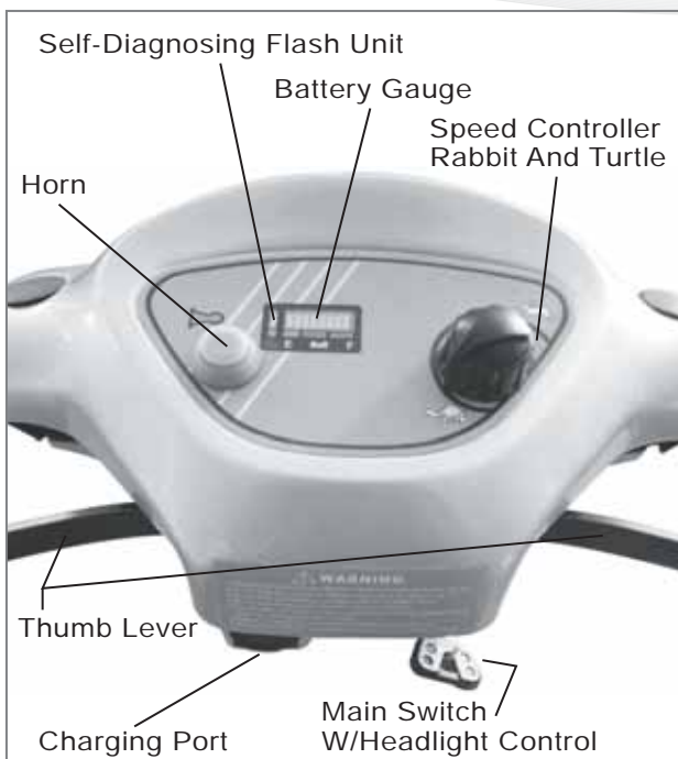
Figure 2 - HS-580 Control Panel
