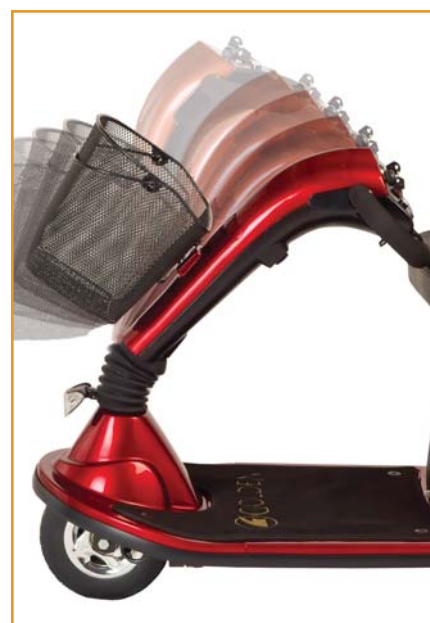
Patented infinite adjustable tiller
