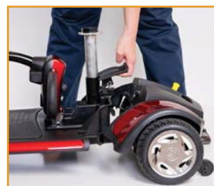
Step 4: Pull up on the drivetrain release lever to separate the front and rear frame sections!
