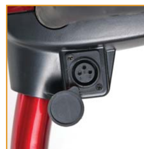
A battery charging port is conveniently located on the tiller under the control panel.
