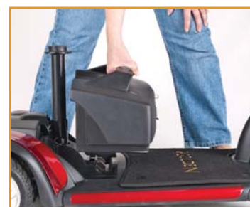
Step 2: Pull out the battery pack!
