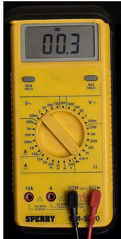
Figure 13. Multimeter (Set to Ohms)
