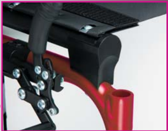
A front capped H-block helps rigidize the frame by holding the seat rails in place.
